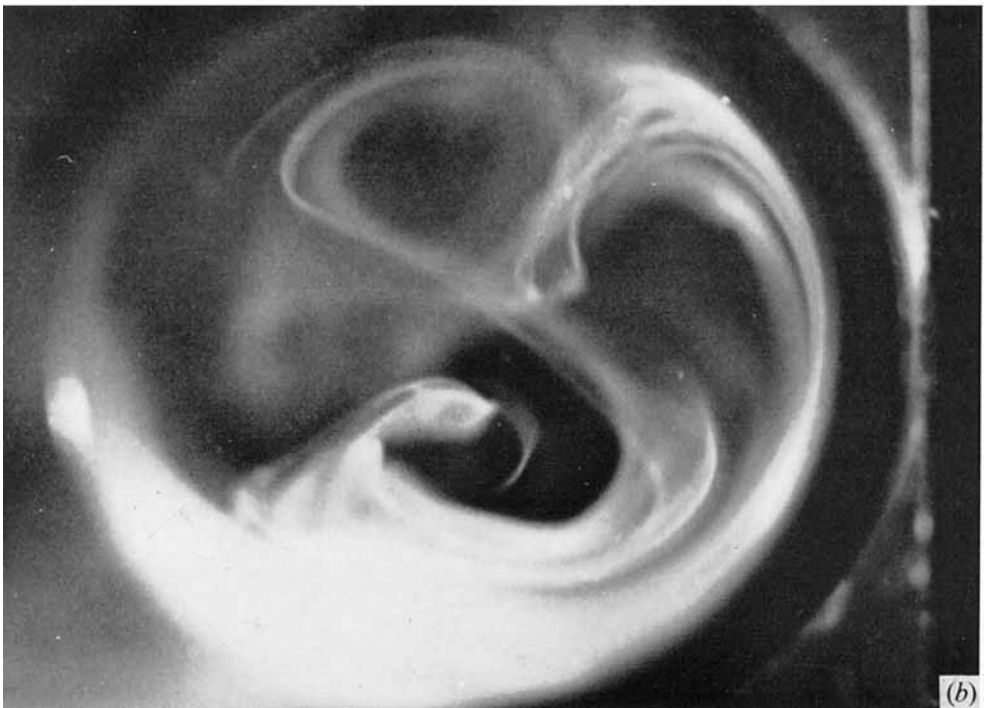
FIGURE 3. (a) End view of a daughter branch of a single junction showing secondary motions when flow is from the parent to the daughters. (b) End view of parent tube of a single junction showing secondary motions when flow is from the daughters to the parent. PEDLEY, SCHROTER AND SUDLOW (Facing p. 384)
